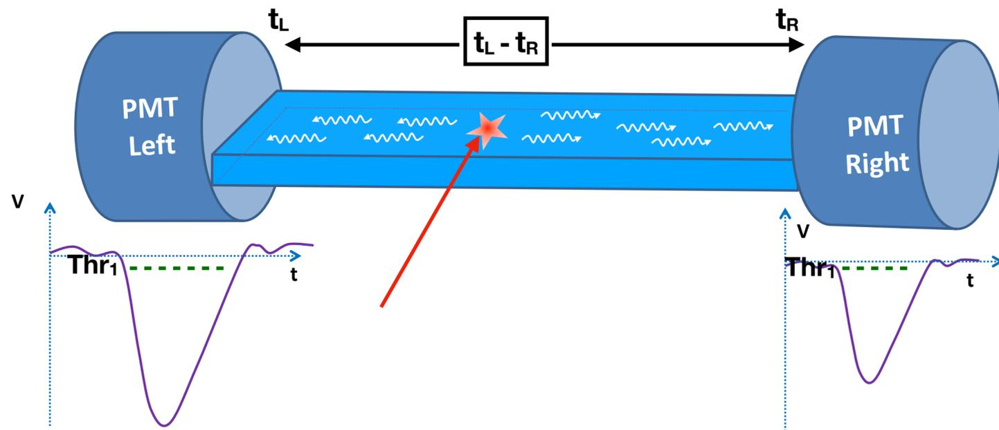
$t_L$  and  $t_R$  refers the time of arrival of light signal at left and right PMT. respectively.
