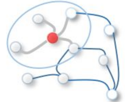
(b) Graph Convolution. To get a hidden representation of the red node, one simple solution of the graph convolutional operation is to take the average value of the node features of the red node along with its neighbors. Different from image data, the neighbors of a node are unordered and variable in size.
