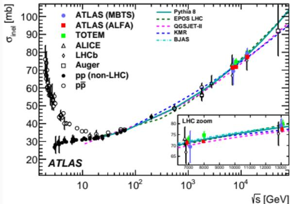
Total inelastic cross section in agreement with previous ATLAS measurements using MBTS detectors
