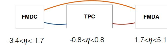
$$v_n\{2\} = \sqrt{\frac{V_{n\Delta}^{\text{TPC-FMDA}} V_{n\Delta}^{\text{TPC-FMDC}}}{V_{n\Delta}^{\text{FMDA-FMDC}}}}$$
